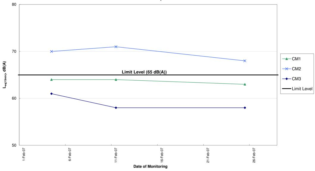
Note: (1) CM2 is a non-façade measurement location. A positive correction of 3dB(A) has been applied to the measured noise level according to EPD's guideline.
