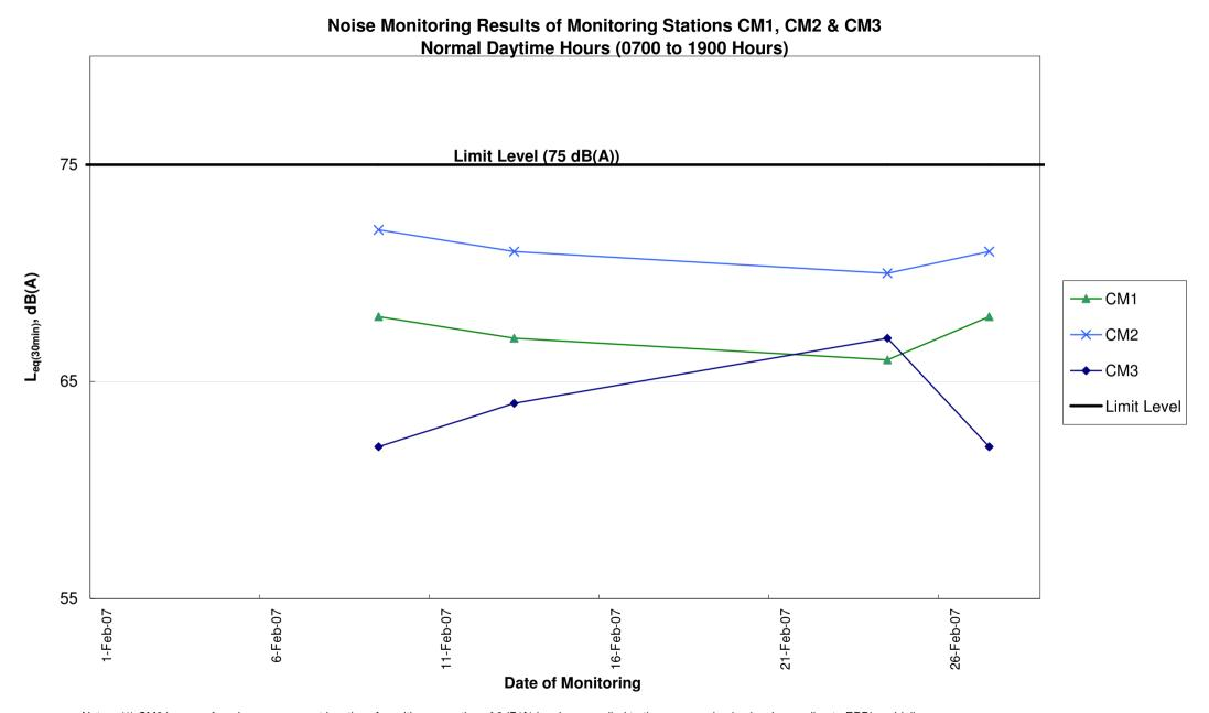
Note: (1) CM2 is a non-façade measurement location. A positive correction of 3dB(A) has been applied to the measured noise level according to EPD's guideline.
